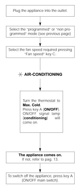
This appliance is fitted with a special safety circuit. When the compressor switches off, this circuit prevents it from switching on again for at least 3 minutes.
